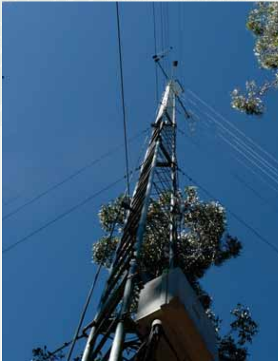
25-m flux tower at Wombat State forest (Victoria) above the canopy of a dry E. obliqua woodland.
