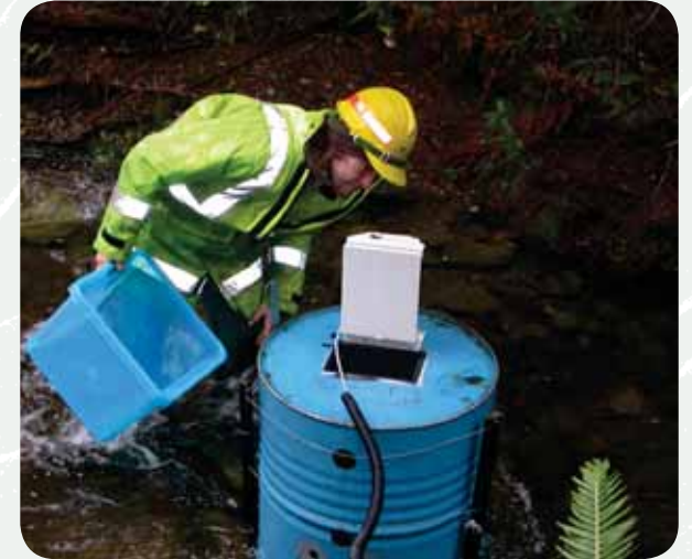
Peter Sheldon inspects a stream-height data-logger at Ben Nevis.
