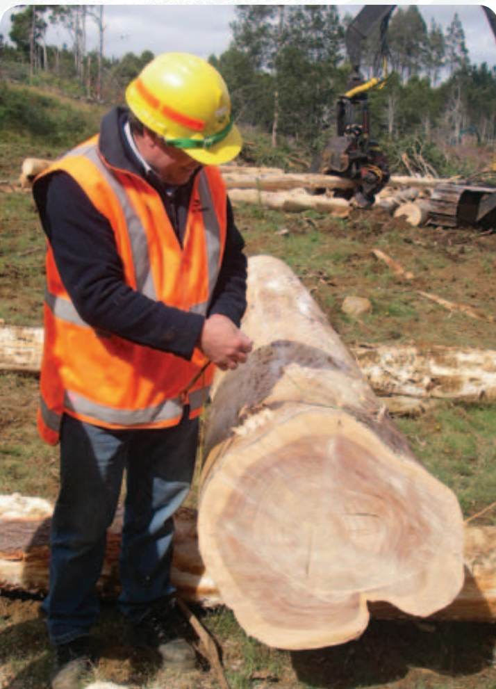
Dr Paul Adams measuring the large-end diameter of a Eucalyptus nitens log which is being used in a processing study with Britton Timbers.
