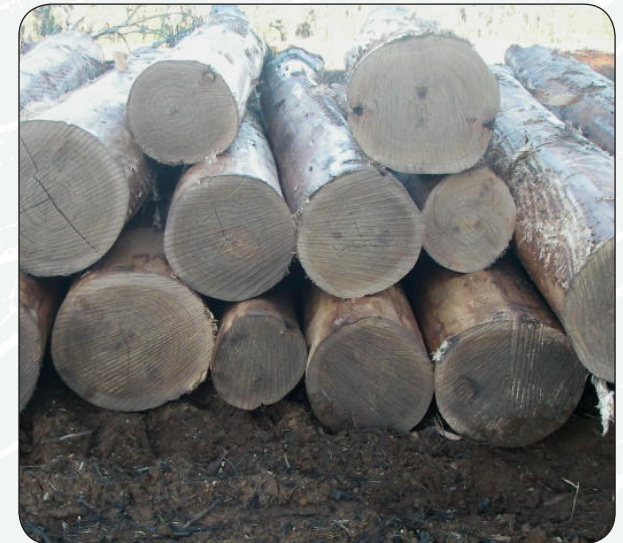
Figure 1. E. nitens pruned logs harvested from the Meunna silviculture trial (aged 22 years). Trees had been 2-lift pruned to 5.4 m and thinned to 200 stems per hectare at age 6 years. Log lengths range from 3.5 m to 5.7 m with small end diameters from 30 cm to 57 cm. Log ends have been waxed to reduce end splitting.
