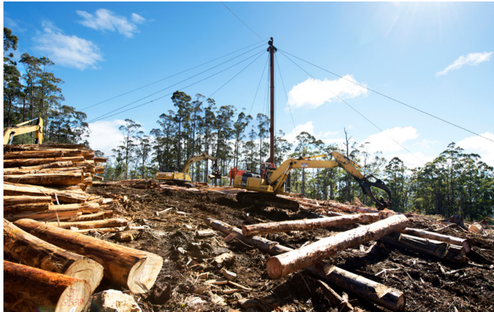
Cable harvesting operation at forest coupe ARO34E in the Arve Valley, Southern Forests, Tasmania.
