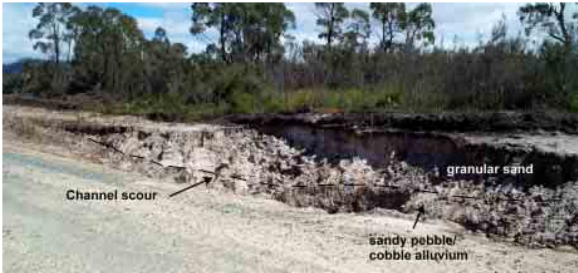
Figure 11: View looking to the southwest of the granular sand lens overlying sandy pebble/cobble facies at site 13, showing scoured surface on which the sand lens was deposited. The sand facies lenses out to both the south (shown) and north (out of photo to the RHS).
