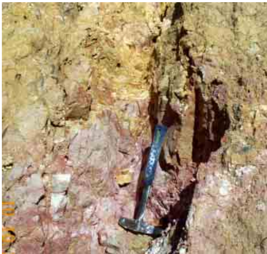
Figure 4: Detail of soft, deeply weathered Permian bedrock at site 18, showing patchy pale yellowish and pinkish-red colours, and fine iron-stained fractures. Visible pebbles are debris from the overlying alluvium.
