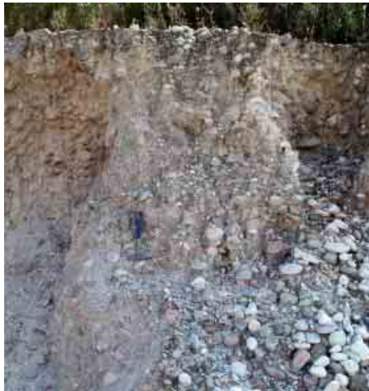
Figure 10: Exposure of over 2.5 metre thickness of sandy pebble/cobble alluvium in a quarry face at site 16, where the unit thickens and descends to lower altitude on the eastern side of the Southwood spur (see figures 13 and 14).
