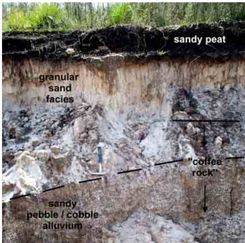
Figure 12: Detailed view of granular sand unit at site 13, showing overlying sandy peat O-horizon, and underlying sandy pebble/cobble alluvium. Hammer handle approx. 300 mm long.
