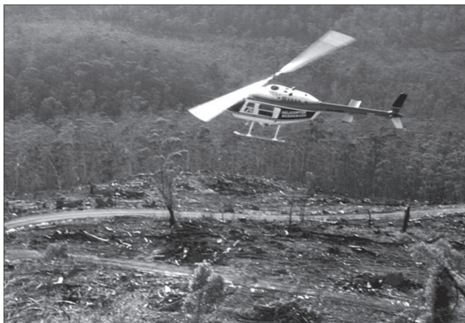
Sowing eucalypt seed on a recently burnt coupe using a helicopter equipped with a Brohm heliseeder unit.
