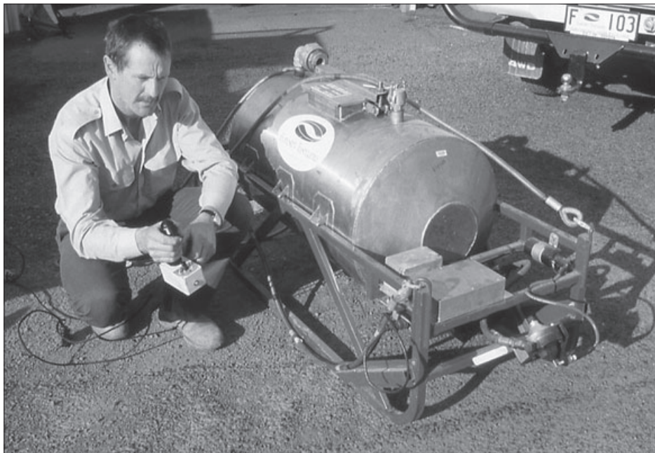
The current helitorch. This is known as the 'Firefly' and is based on a New Zealand design. It is lighter and uses an electrode to provide a continuous spark which ignites the gel as it passes. (Rod McNeill, Aerial Operations Officer in the 1980s and 1990s.)
