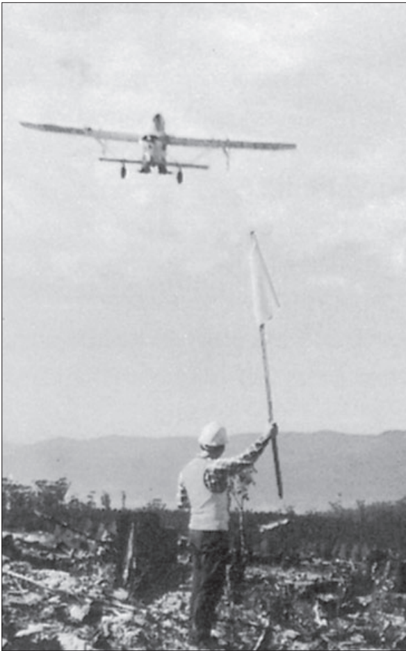
The early ground-based method of marking aerial sowing runs using flag wavers. This method was abandoned when on-board aircraft guidance systems became available.
