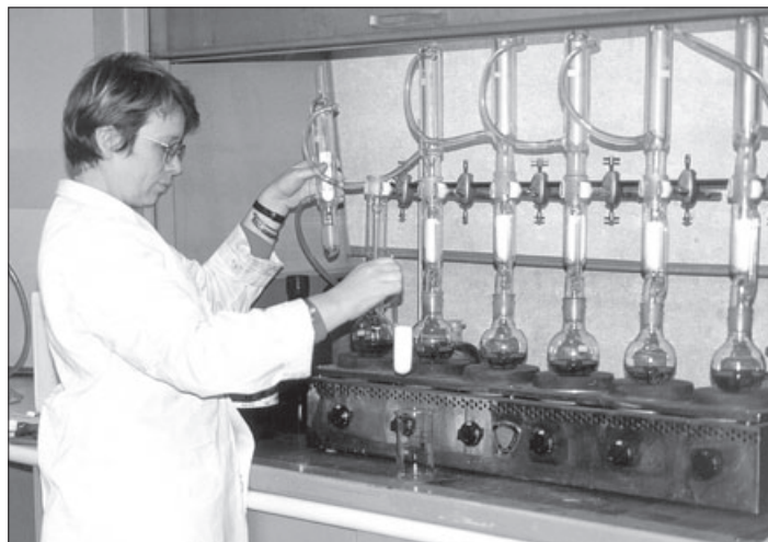
Above: Measuring the extractives content of wood samples – part of a study examining the genetic variation of wood decay in Eucalyptus nitens , 2000. (Jacinta Lesek pictured.)
