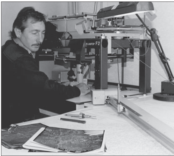
Using a Planitop plotting machine to produce forest type maps. (Tim Madden, operator.)
