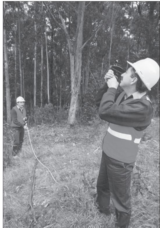
Measuring tree heights in the forest to check those determined from aerial photographs. (Tim Madden, left, and John Gardner.)
