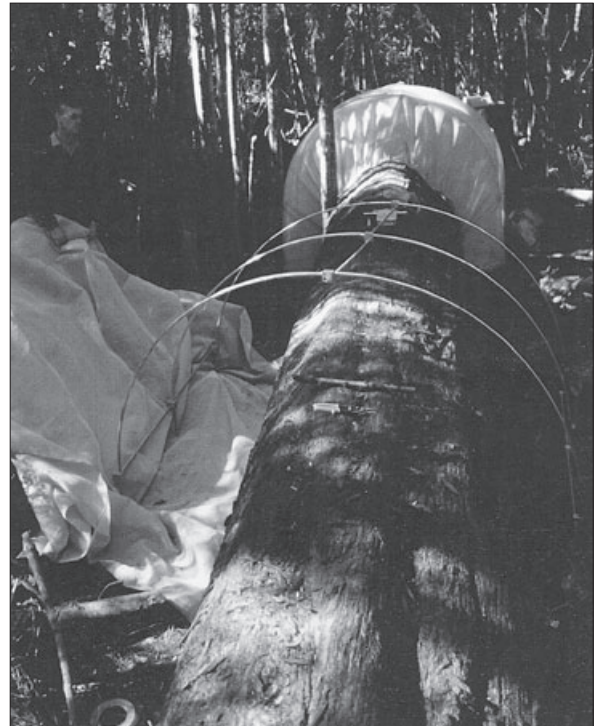
Construction of an emergence trap in the log-decay project, showing the aluminium frame and shade-cloth tent.
