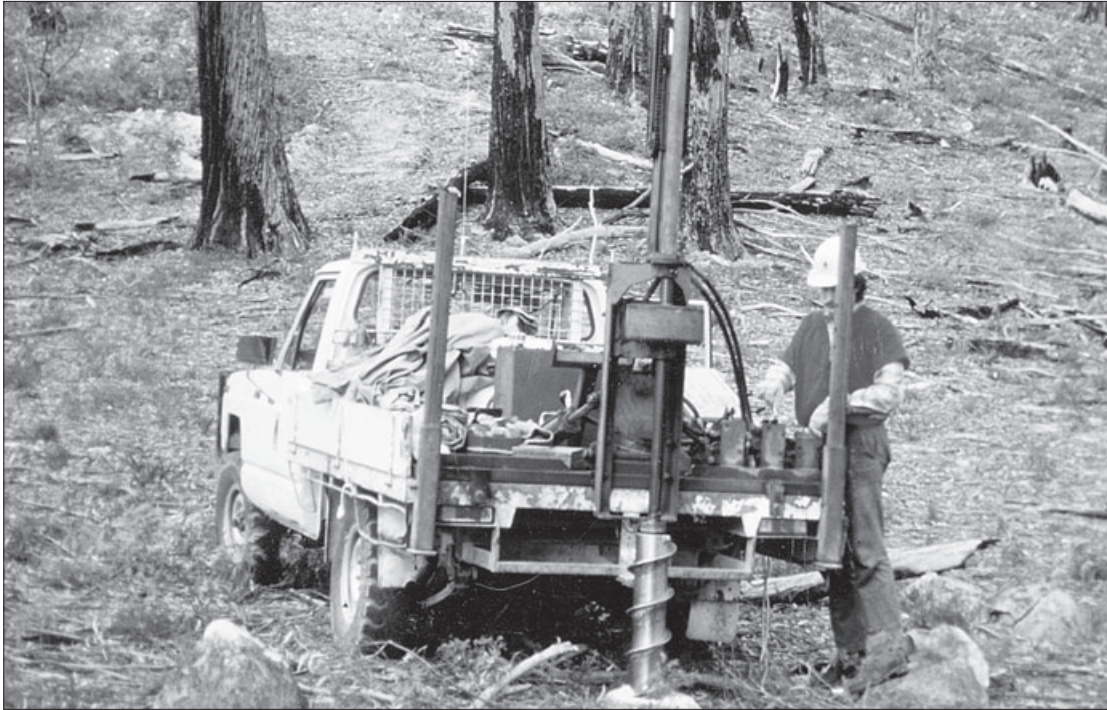
John Grant using a truck-mounted hydraulic auger to sample granite soils in the survey site near St Helens.
