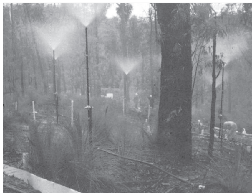
Simulating high rainfall in an experiment in the north-east to assess its effects on granite soils.
