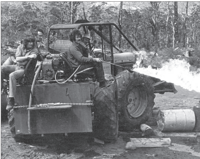
Testing a flame thrower mounted on a tractor, 1971. The tank contained a petrol/diesel mixture which was ignited by being pumped past a pilot flame in a wick. (At rear of tractor, Gary Siely, left, and Mark Whitney; others unidentified.)
