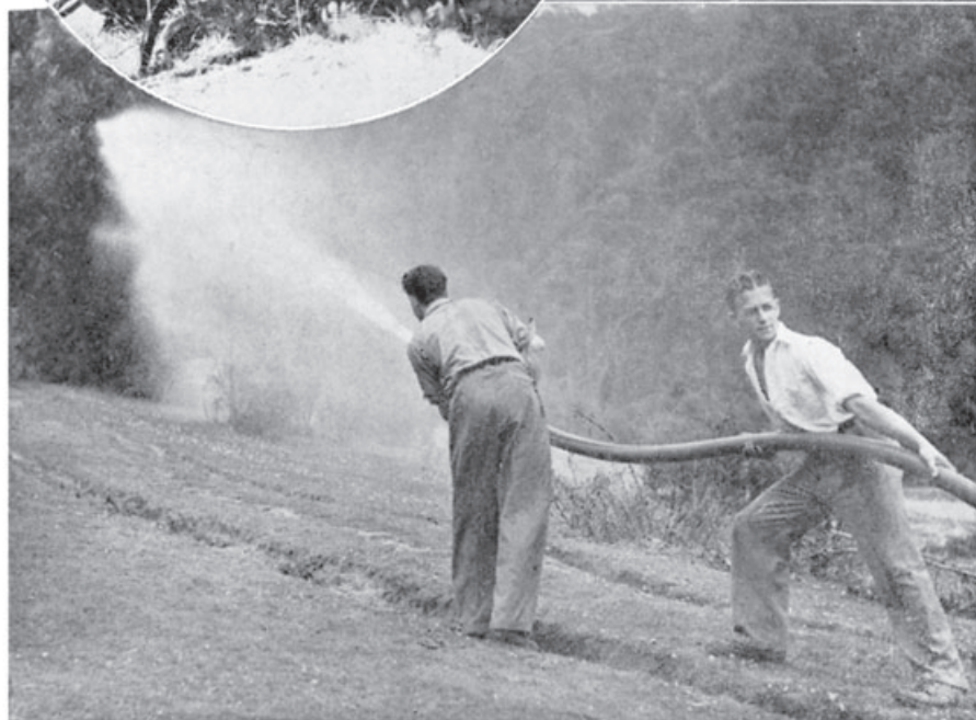
Details of the Dennis Pump taken from the Forestry Department's 1938-39 Annual Report. The collection of photos is entitled 'A Dennis Fire pump in action', with the caption for the bottom photo given as "The hose in action, throwing a jet of approximately 100 feet".
