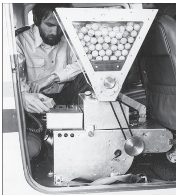
An early version of the aerial incendiary machine. The ping-pong balls were fed from the hopper into a gate where they were injected with glycol; they then dropped from a chute and were alight before hitting the ground.
