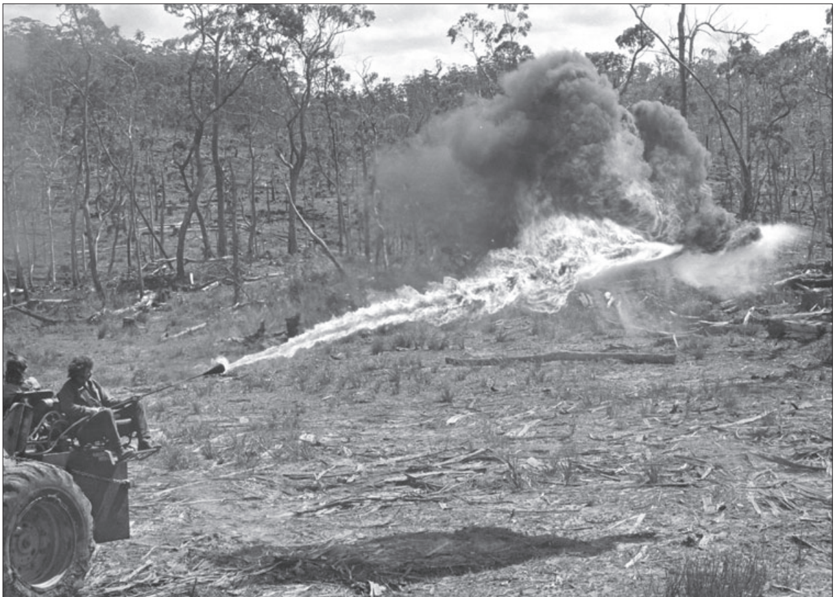
Test-firing the flame thrower in dry logging slash on the east coast.
