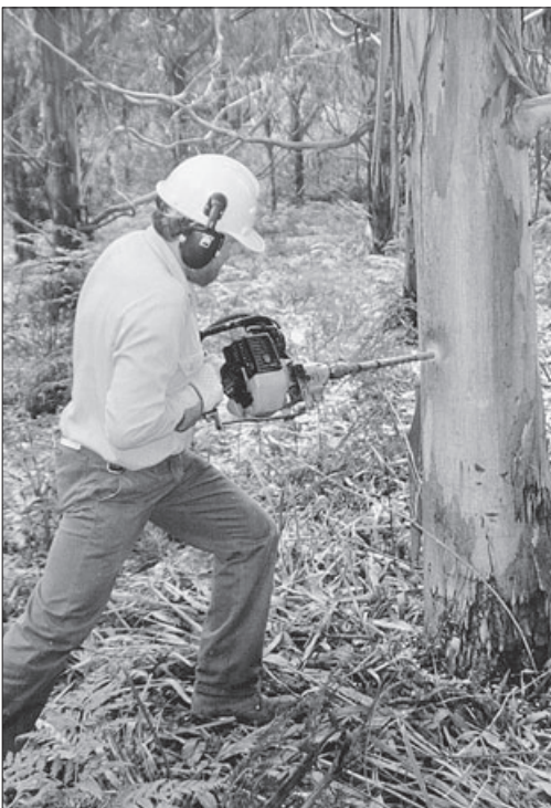
Above: Measuring the extractives content of wood samples – part of a study examining the genetic variation of wood decay in Eucalyptus nitens , 2000. (Jacinta Lesek pictured.)
