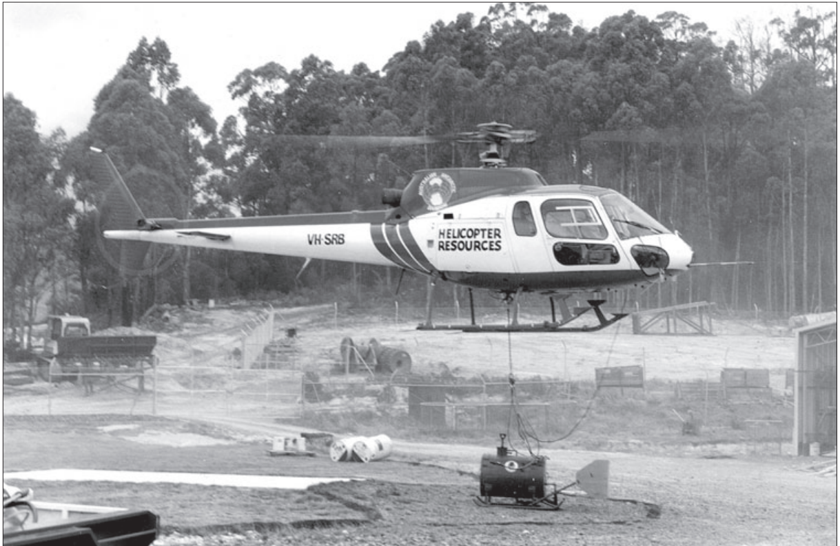
The first helitorch used in Tasmania. It was based on a Western Australian design, comprising a welded steel pressure vessel with a propane gas lighting system to ignite the petrol gel.
