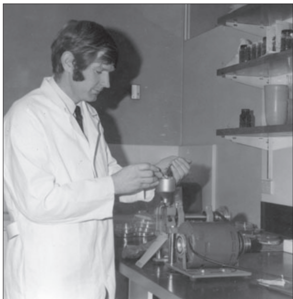
Grinding radiata pine needles for analysis, as part of trials testing responses to fertilisers in 1972. (Bill Neilsen pictured.)
