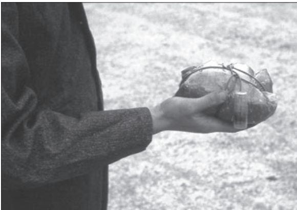
A gel blivet used in trials of remote ignition at Maydena in the late 1960s. This was an early prototype exploding package, containing petrol gel with a small cordtex fuse and a detonator wrapped around with plastic igniter cord.
