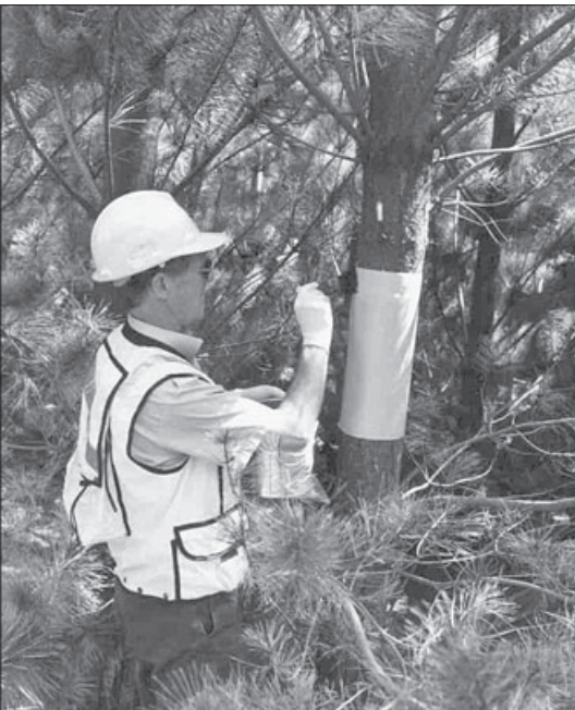
A sticky band trap being installed by Dick Bashford on a pine tree to monitor the occurrence of exotic pests in high-risk areas surrounding ports.
