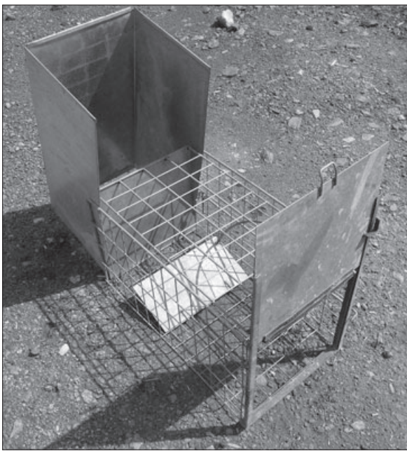
The Mersey Box Trap — a very effective trap for catching browsing animals, developed by Mersey District staff.
