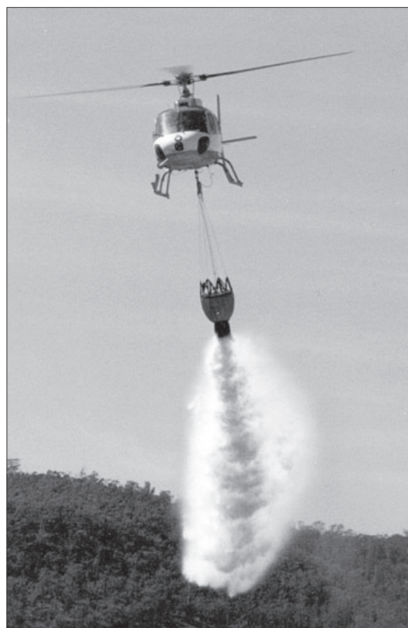
A Squirrel AS40B helicopter dropping a water/foam mixture from a collapsible bambi bucket during trials near Craigebourne Dam, south-eastern Tasmania.
