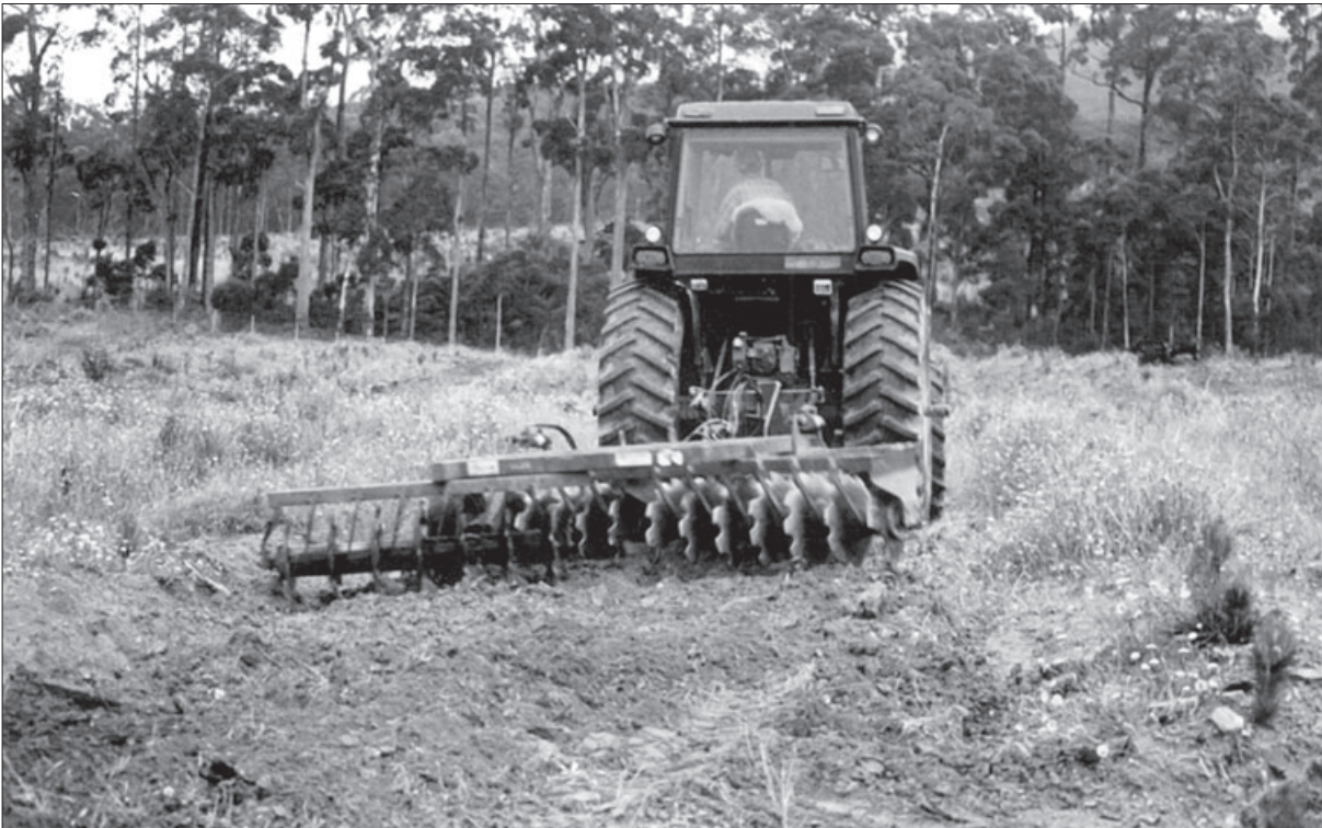
Cultivating between rows of six-month-old pines to control weeds, using tractor-drawn discs, c. 1996. Post-planting weed control in plantations was one of the more successful techniques introduced as an alternative to the use of chemicals.
