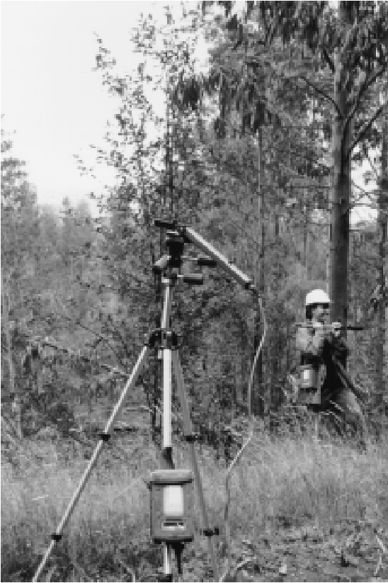
Photo 1. Note the sensor mounted on the tripod in the clearing and the data logger recording incident radiation. The second sensor is carried by the operator, as shown, for below canopy measurements.
