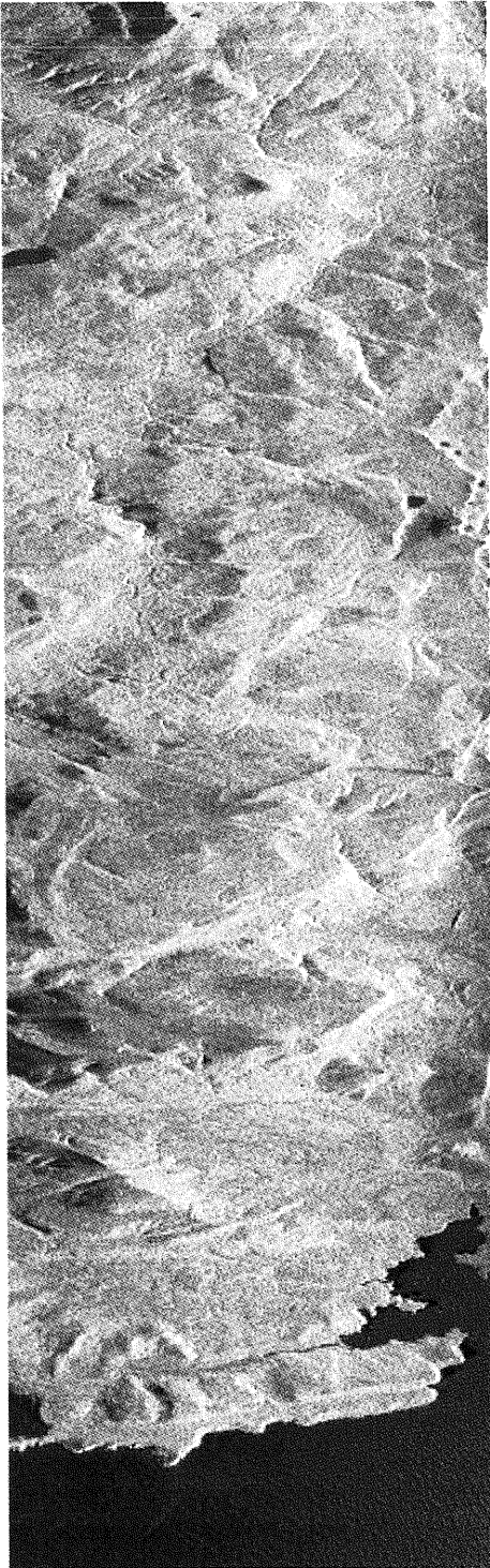
Figure 3. Quick-look print from the NASA Jet Propulsion Laboratory of the PACRIM-2 AIRSAR campaign over Warra. The transect is uncorrected RADAR backscatter covering a 60 km swath of southern Tasmania.
