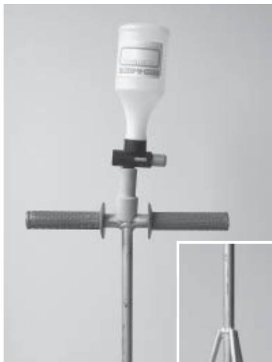
Photo 1. The spot sower. Above: upper part of the spot sower showing the seed dispenser. Right: base of the spot sower showing the scarifying device and the hollow tube through which the seed falls.
