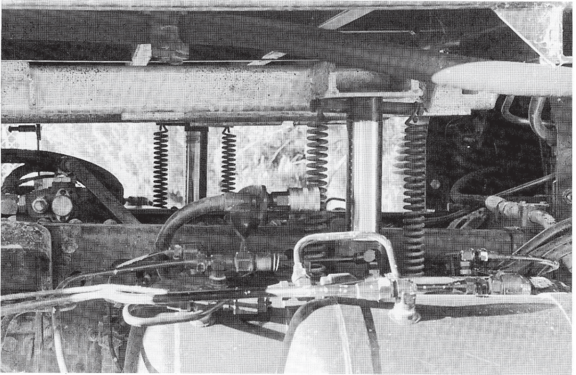
Photo 3. The module is lifted from the truck chassis by single-acting hydraulic rams.
