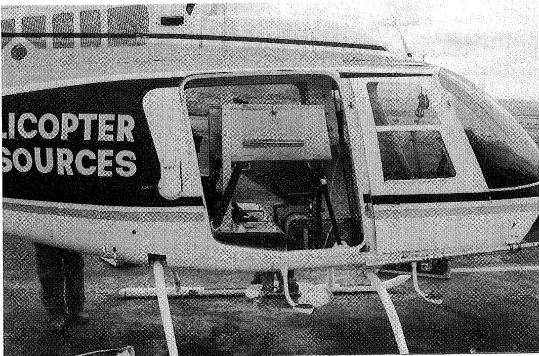
Photo 5. Heliseeder equipment installed in Bell 206 helicopter.
