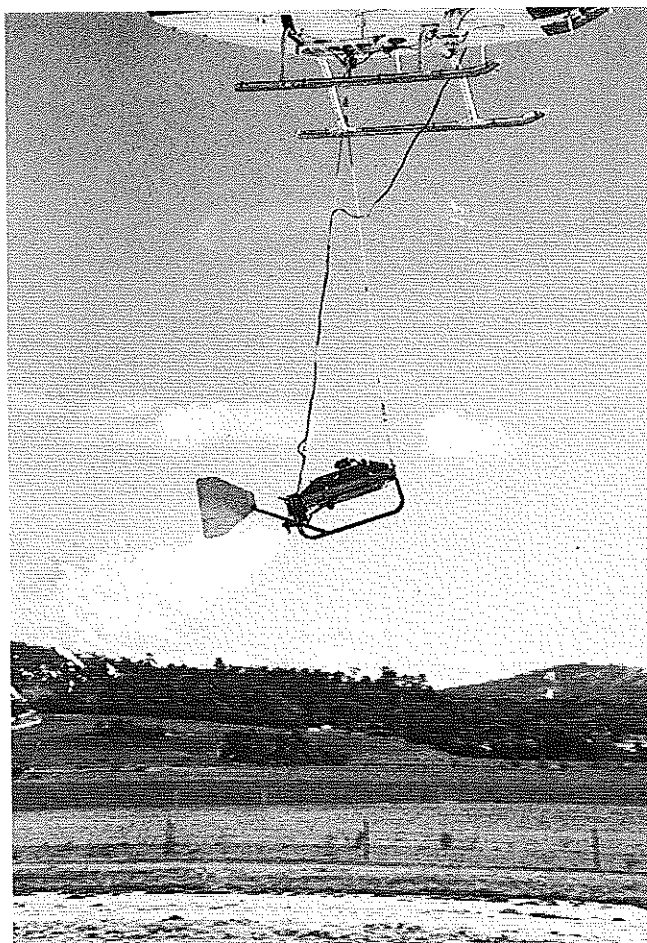
Photo 1. The aerial drip-torch delivering burning gel for aerial ignition operations.
