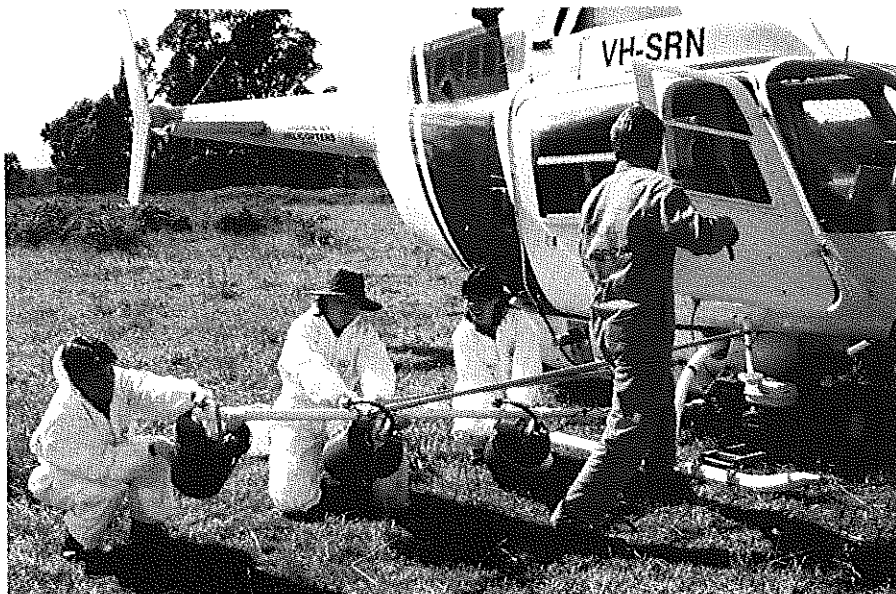
Photo 6. Measuring the flow rate of the biological insecticide Novodor. The helicopter is fitted with six Micronair AU-5000 rotary nozzles which deliver the insecticide to the plantations.
