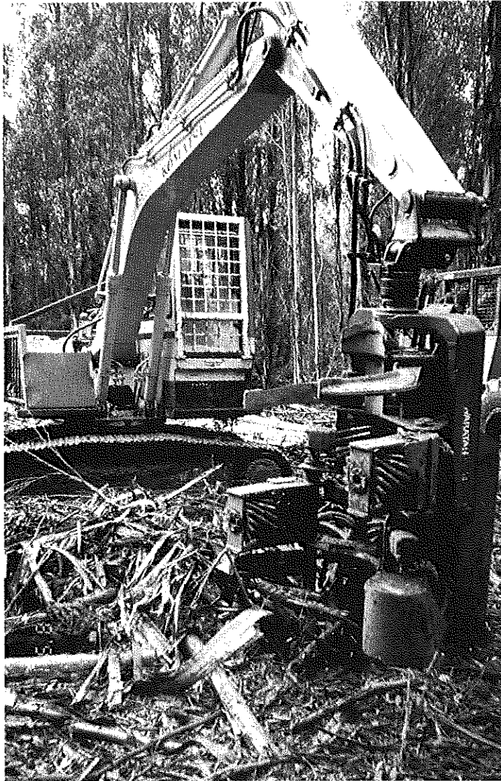
Photo 5. An excavator fitted with a Waratah felling and processing head was used to speed the debarking process and increase production in the ground-based thinning operation.
