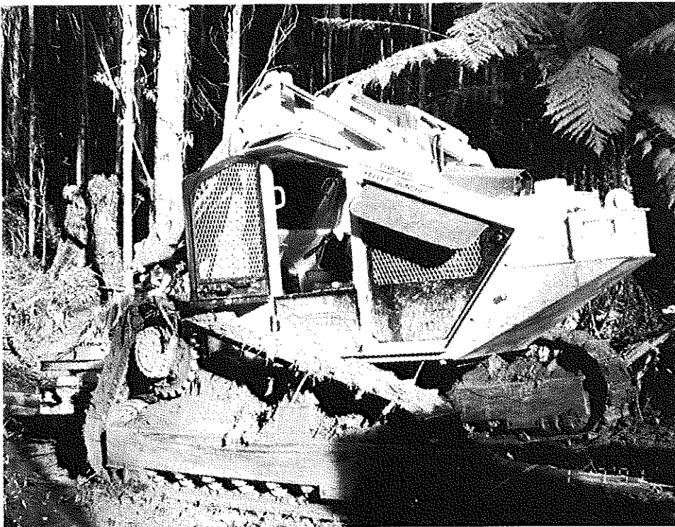
Photo 4. The Bell tracked feller buncher used for felling during ground-based thinning operations.
