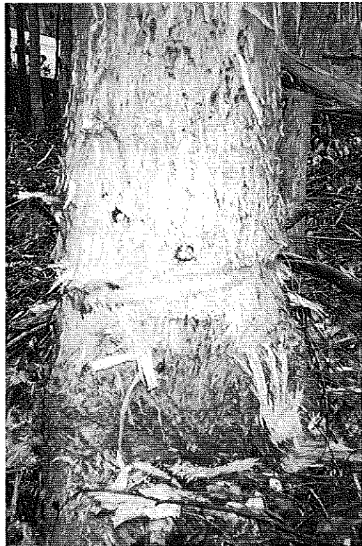
Photo 8. In early trials with cable thinning, injury to the tail-hold tree was caused by rope-burn from the steel cable used for the skyline. This problem has now been eliminated using broad-band strapping.
