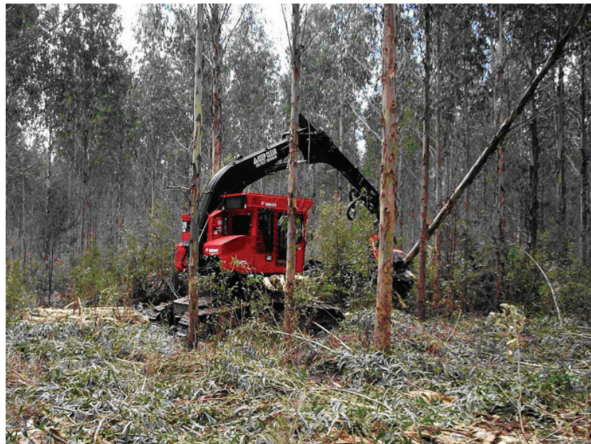
Figure 3. Thinning a eucalypt plantation in Tasmania using modern equipment; such machines ensure minimum damage to both the harvested and the retained stems.
